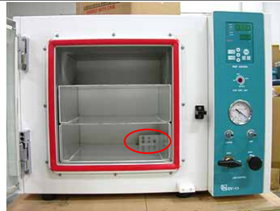
The circled is Temperature control Sensor
